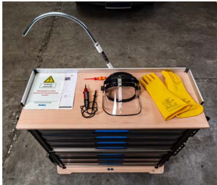
Mobile high-voltage workplace
