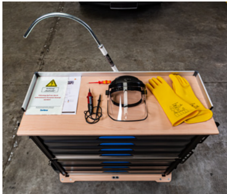
Mobile high-voltage workplace
